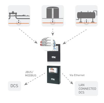
In the event of hydrocarbon leakage, the sense cable in contact with the liquid detects and transmits rapidly the location of the leak to the monitoring
