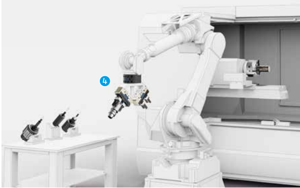
Loading of a machine tool with a jointed-arm robot
