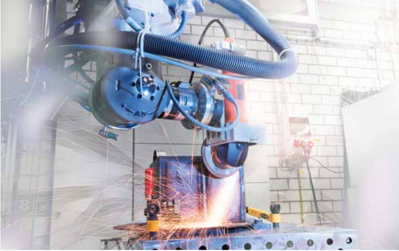
Automated grinding of supply air chambers for stoves
