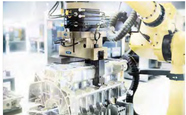
Handling of motor blocks
