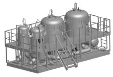
Filtration/separation and fuel conditioning equipment to assure clean, dry fuel that meet the latest specifications.
