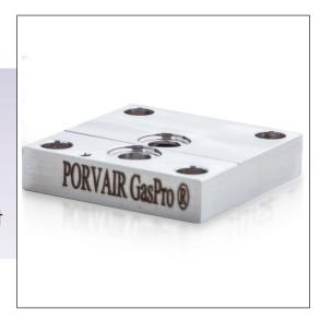
GasPro™ TEM-737125 is a unique filter for surface mount gas delivery systems, designed to be placed under another component. Placing under a valve or regulator eliminates one substrate and effectively shortens the system and reduces its cost.
