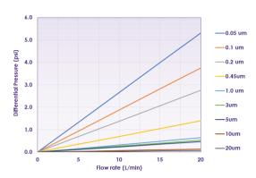
\*Flow rate is for a 25.4 cm (10 in) cartridge. For liquids other than water, multiply differential pressure by fluid viscosity (cP).
