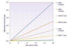
\*Flow rate is for water at 20°C through a 10 in cartridge. For liquids other than water, multiply differential pressure by fluid viscosity (cP).
