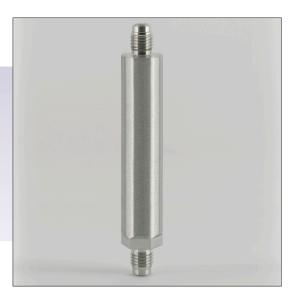
GasPro<sup>™</sup> TEM-1900 Series filters are designed for 3 nm particle retention up to flow rates of 100 slpm and temperatures of 121°C (250°F).
