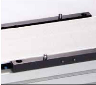
Two locating dowel pins shown in carriage
