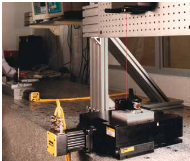
ZP200 utilized in a laser test set-up
