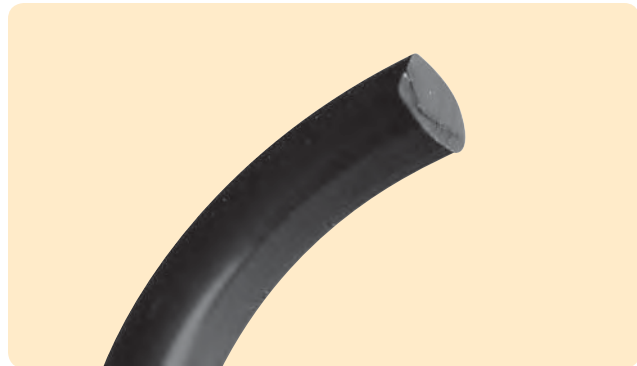
Figure 10-5: Wear is Seen as Flattening of O-ring on One Side
