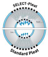
SELECT pleating provides an optimized effective filtration area, dramatically increasing flow rates compared to products with standard pleat format.
