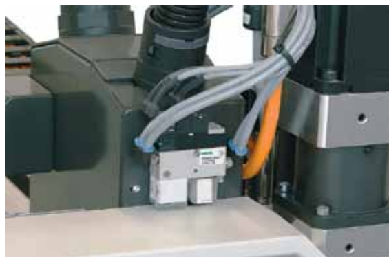
Central vacuum generation by compact ejectors NSCPM
