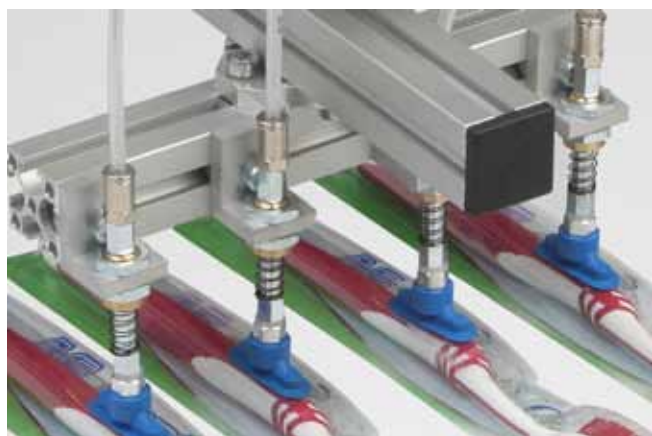
Flat suction cups NSGON being used for handling blister packaging
