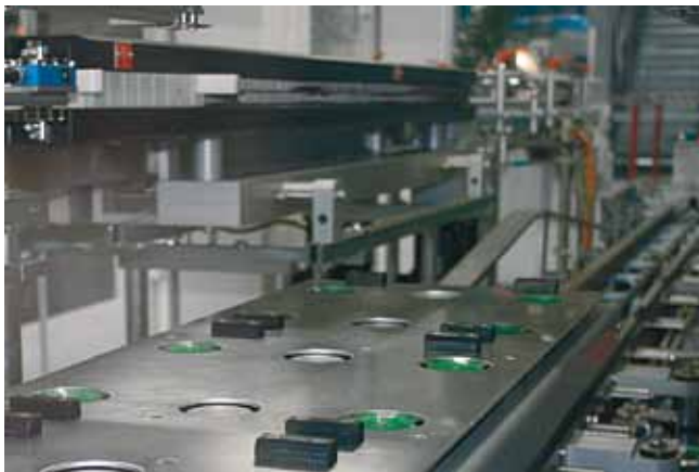
Flat suction cups NSPFX being used in packaging machines
