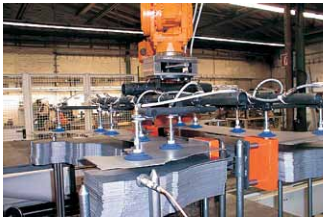
Mounting example spring plungers NFSTE
