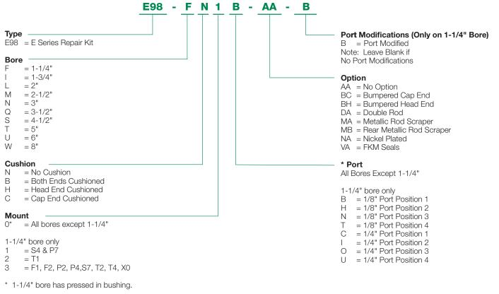
**Note:** Options listed are ones that apply to a repair kit only. Model number is set up to use option code supplied with original cylinder or with any above.
