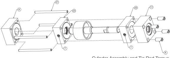
Cylinder Assembly and Tie Rod Torque
