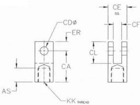
Pivot Pin for Rod Clevis
