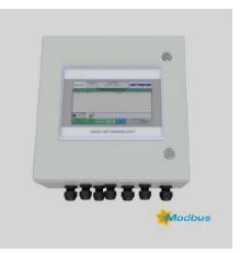
FLD-TSP7 provides power and multiplexed communications through the Naftosense ERBUS proprietary bus resulting in a lean communication infrastructure. The FLD-TSP7 has a high-level interfacing to DCS/SCADA is implemented through the RS-485 serial output with Modbus RTU, or through dry contacts. With options for up to 9 SPDT relays, alarms, and communications are easy to configure with the FLD-TSP7.
