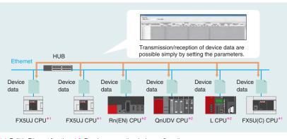
\*1: Built-in Ethernet function \*2: Requires connecting device configuration.
