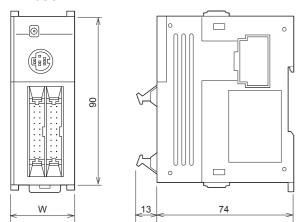
External color: Munsell 0.08GY/7.64/0.81 Unit: mm 35 mm width DIN rail can be installed
