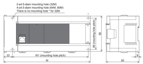
External color: Munsell 0.6B7.6/0.2 Unit: mm The terminal block uses M3 terminal screws 35 mm width DIN rail can be
