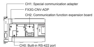
[Configuration example 2] Using two special communication adapters
