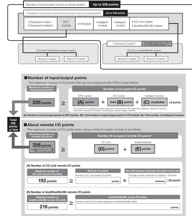
\*: CC-Link IE Field Network Basic remote I/O stations are not calculated as remote I/O points.
