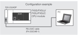
(2) Connection with the RS-232C port attached to PLC (using FX5-232-BD)
