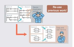
• In program (processing) management, programs can be easily diverted by dragging & dropping FBs.
