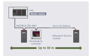
• FX5 CPU module can connect, as a master or slave station of MODBUS communication, to various MODBUS communication devices.
