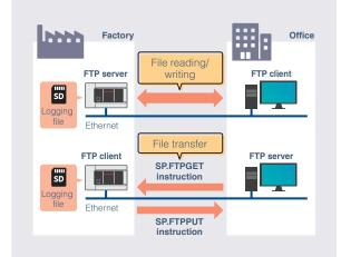
Using the file transfer function instruction, you can transfer logging files, etc., and obtain data from the server without complicated settings and operations in the upper system (FTP server).
