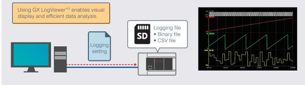
• Logging data collected from CPU modules can be displayed visually for efficient data analysis.
