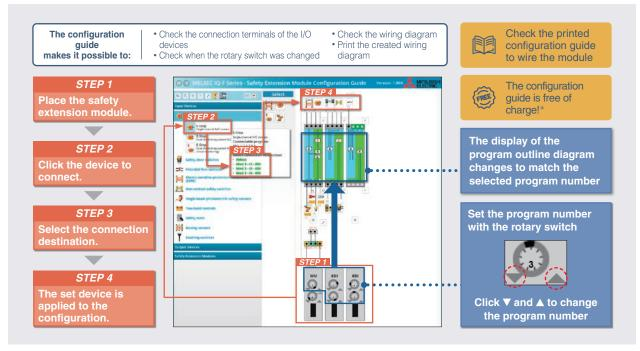
• Easily check the system configuration, settings, and wiring of the safety extension module.
