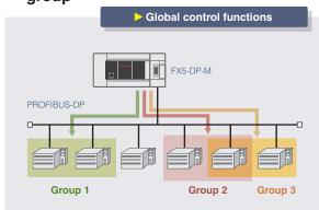
The global control function allows for synchronous communication of input/output data for each designated group through multicast communication (simultaneous broadcast communication).
