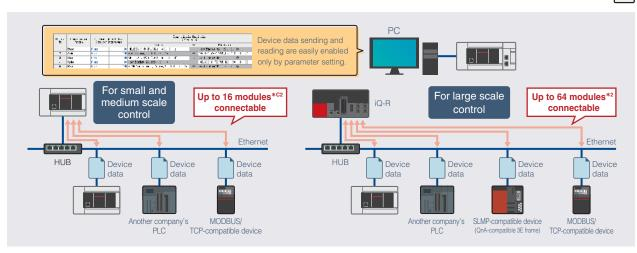
• Using a simple parameter setting with GX Works3 as the master, device data such as production data can be transferred without a program.
