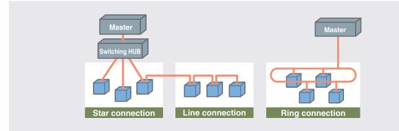
• Connection formats, such as highly reliable ring connection or simple line connection, can be selected based on installation cost.
