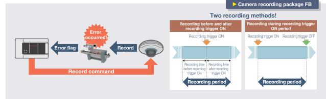
• Video of operating conditions when errors occur can be saved for use during error analysis.
