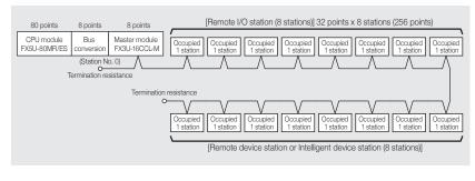
The maximum number of remote I/O stations to be connected is 8 when connecting 80-point type CPU module and FX3U-16CCL-M. The maximum number of remote I/O stations to be connected is less than 8 when the total number of points exceeds the maximum I/O points (512 points) due to the connection of I/O modules and intelligent function modules.
