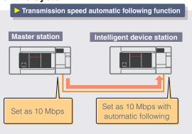
· When used as an intelligent device station, the transmission speed can be set to automatic following. The transmission speed automatically follows the transmission speed of the master station, preventing setting errors.
