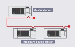
• The FX5-CCL-MS module is equipped with both the master station function and the intelligent device station function, and can be used as either station when switched by a parameter.
