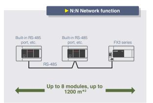
In this communication, a connection is set up with the FX5 PLC or FX3 PLC through RS-485 communication to automatically exchange data.
