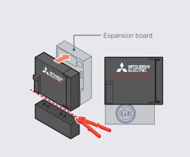
• The cover can be cut off and attached to the upper section of other expansion boards.
