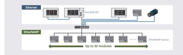
• It can seamlessly communicate with EtherNet/IP networks using the CIP communication protocol. EtherNet/IP and general-purpose Ethernet communication can coexist.
