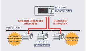
• Using the buffer memory makes it possible to obtain communications error information or extended communications error information generated by a slave station during I/O data transmission.
