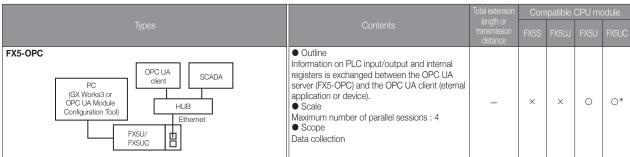
\*: Connection with FX5UC CPU module requires connector conversion module (FX5-CNV-IFC) or extension power supply module (FX5-C1PS-5V).
