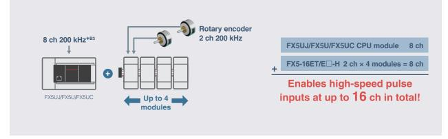
• The number of channels used for high-speed counters can be increased.
