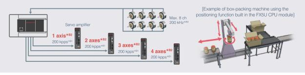
• Positioning function is built into CPU module (transistor output type only).
