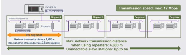
• The MELSEC iQ-F series can be connected as a master station for PROFIBUS-DP networks.
