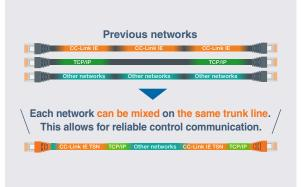
No need to configure every network! Since TCP/IP communication can be mixed on the same trunk line, a single network can be used.
