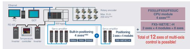
• Further multi-axis control is possible by adding to the FX5UJ/FX5U/FX5UC CPU module.
