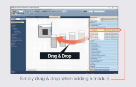
• With GX Works3, the module configuration diagram can be created by dragging and dropping selected parts.
