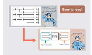
• In FB, only the necessary input/output are displayed, so the appearance is simple and programs are easier to read.
