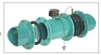
**Plastic or internally coated pipe** - Grounding rings can be installed to establish a connection to earth ground See the Ultra Mag IOM Manual, Lit. # 30119-03, for more information on grounding configurations using grounding rods and grounding rings.
