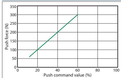
Correlation diagram between push force and push command value
