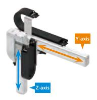
For this type, the base of the Z-axis (vertical axis) is fixed to the Y-axis slider with the Y-axis side-mounted. The Z-axis slider moves vertically, allowing mounting of jigs or chucks for transport, raising, or lowering of workpieces.
