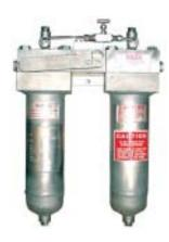
HILCO Hyflow duplex filters provide continuous flow during fluid transfer and cartridge changeout. An integral transfer valve with two stops and a witness mark indicates the side of the filter in use. In-line filtration of fluids up to 3,000 PSIG, ASME Code and non-Code, with flow rates to 75 GPM is possible with these filters. HILCO duplex filters are ideal for cost effective, efficient filtration of fuels, solvents, hydraulic, lube and compressor oils.
