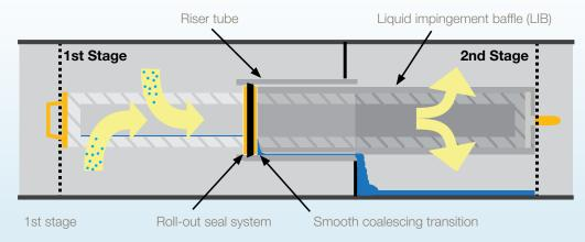
**STANDARD RECIPE:** 99.99% of 0.3 micron & larger solid particles 99.8% of 0.3 micron & larger liquid droplets < 50 PPB (wt) effluent
