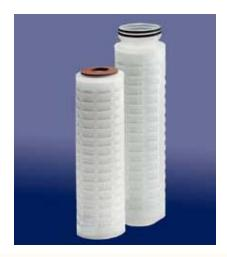
Extended life and absolute retention efficiency make the Clariflow<sup>®</sup> Wine product an ideal filter for the clarification of wine. At the heart of this design is a special membrane composed of polyethersulfone (PES). Choosing either the 0.65 or 0.45  $\mu$ m pore sizes for red and white wines, PES membrane offers superior flow, extended on-stream life, and the consistent removal of microorganisms and particulates.
