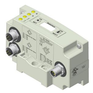
The following graphic displays represent the main menu selections of the 580 PROFINET<sup>™</sup> communication (node). Use the NEXT button to scroll through the Main menu headings shown below. At this level pressing the SET button allows access to the Sub-Menus. Please see the appropriate pages referenced below for further details and descriptions of the Sub-Menus. *NOTE: WHEN A NETWORK I/O CONNECTION IS ESTABLISHED, MANUAL CHANGES TO NODE PARAMETERS ARE NOT ALLOWED!*
