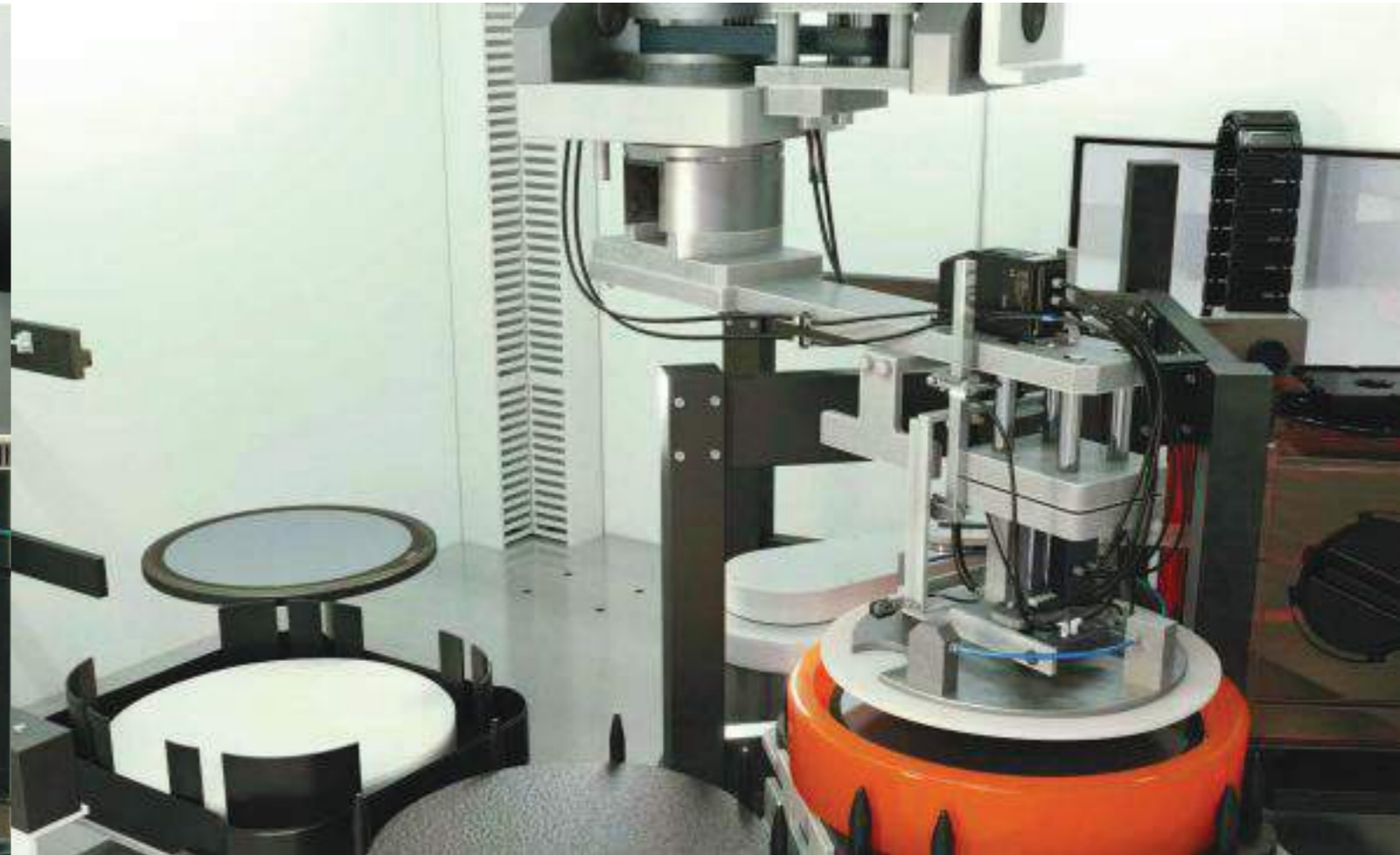
Photoelectric sensors attached to the robot in the packaging equipment are used to identify the presence of wafer buffers.
