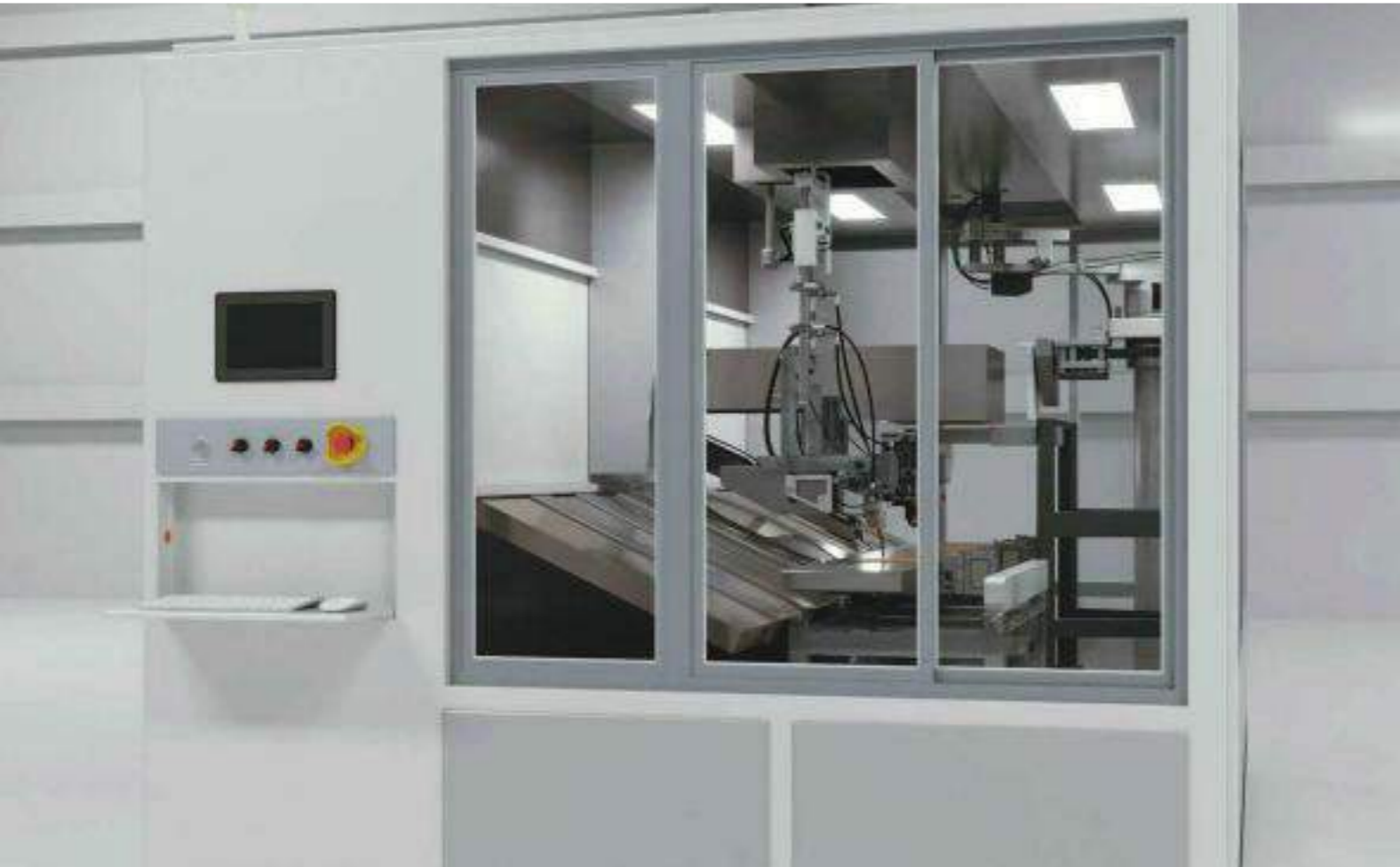
Emergency stop button switches can be used to manually stop operation of the equipment before opening the door.
