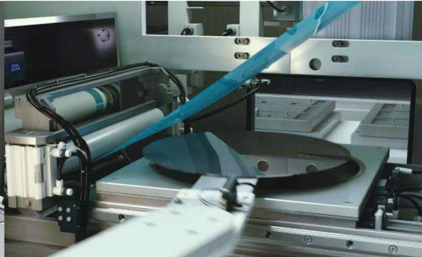
Fiber optic amplifiers are used to check the received light amount depending on the presence of wafers and transmit control signals.
