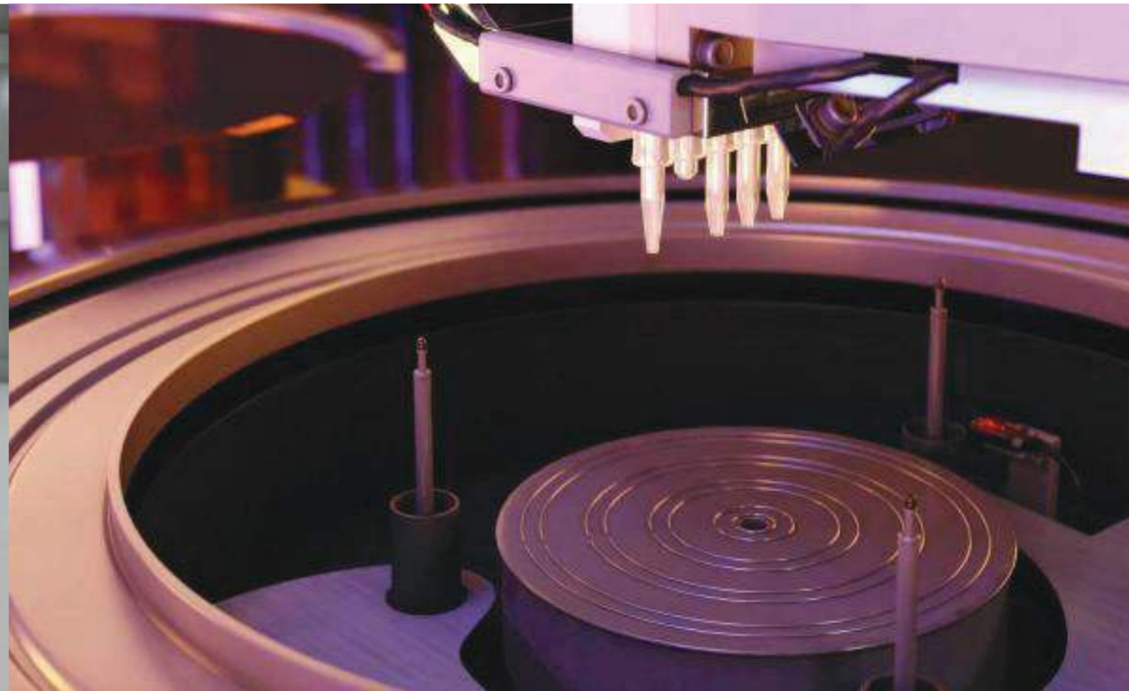
Photoelectric sensors located at the bottom of the spin coaster are used to detect whether wafer is mounted before applying the solution.
