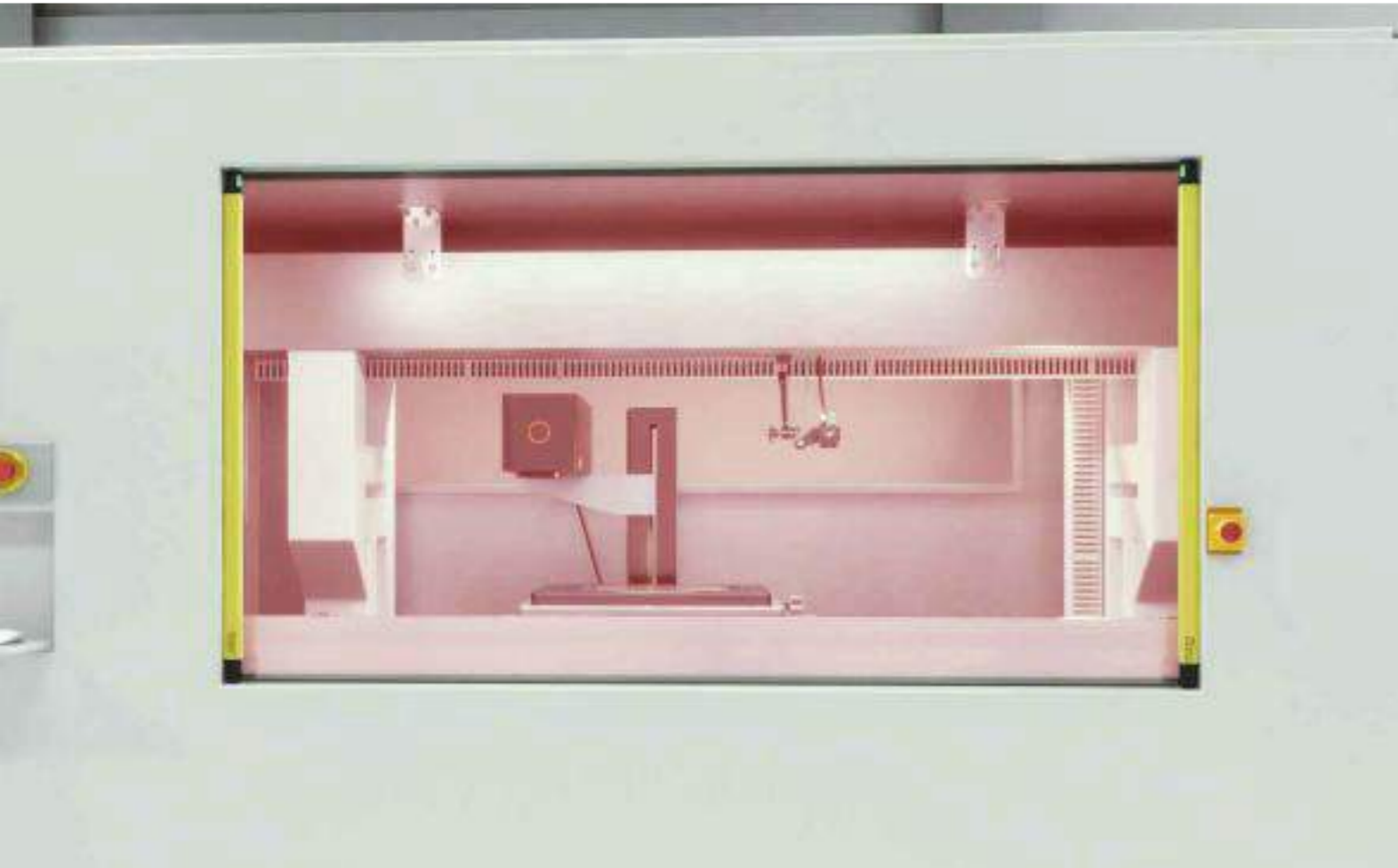
Safety light curtains can be used to detect human access to hazardous areas while equipment is operating.
