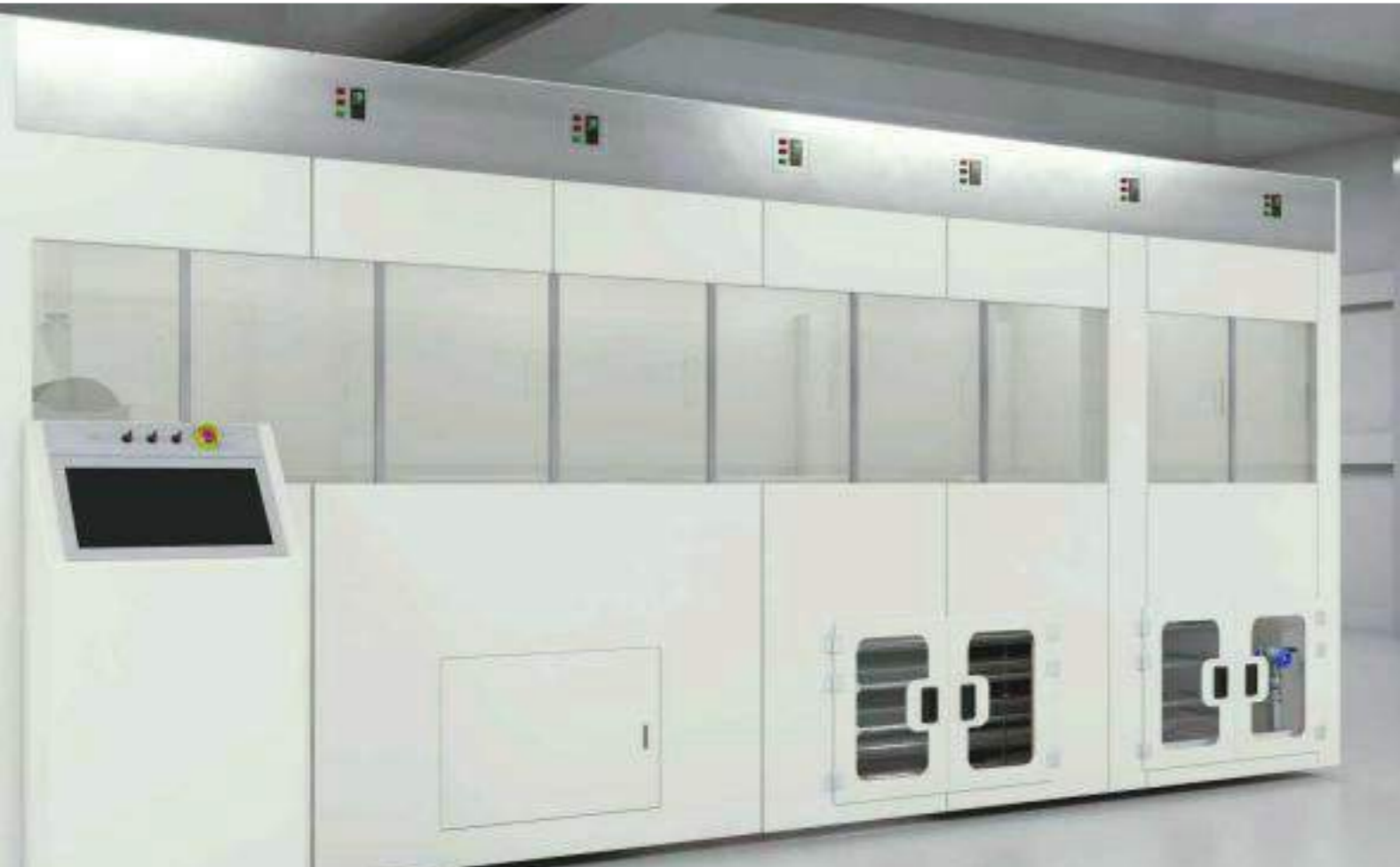
Temperature controllers are used to control the temperature of the cleaning solution in the equipment for cleaning foreign substances or oxide film.
