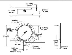
100 mm lower back connect - case mounted U-clamp
