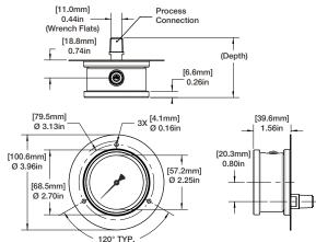
63 mm center back connect **Connection Code Process Connection** Depth 01 1/8 NPT 2.36 [60.0] 02 1/4 NPT 2.50 [63.4] 13 G¼ B 2.49 [63.3] 41 M14x1.5 2.53 [64.3] JIC #4 EJ 2.44 [62.0] JP 2.60 [66.1] 1/4 Tube JR 3% Tube 2.73 [69.4] JS 1/2 Tube 2.86 [72.7] KA 1/4 BSPT 2.42 [61.4] RW SAE 7/16-20 2.60 [66.1]
