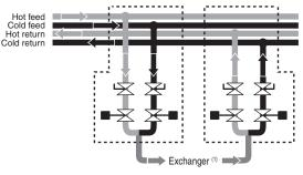
(1) Provide for a unit of two valves for the feed loop and the return loop.
