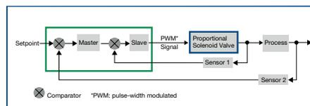
Cascade control helps to significantly increase process quality, by compensating for all the influencing factors and disturbances in the control chain. The valve manages any physical variable that can be influenced by air or an actuator.
