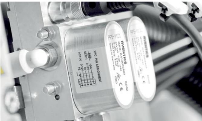
Proportional technology replaces on/off control devices that require larger manifolds. ► p11
