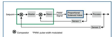
Cascade control enables compensation for disturbances in control chain, improving quality of final products and reducing rejects. ► p15
