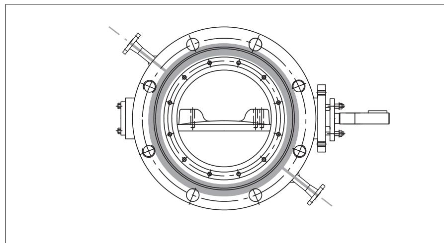
For applications requiring constant higher temperature levels, the L6 valve can be equipped with steam jacket to prevent e.g. liquid sulphur to crystallize. The bearing area is protected by an O-ring to prevent contaminant particles from entering the bearing and packing area.
