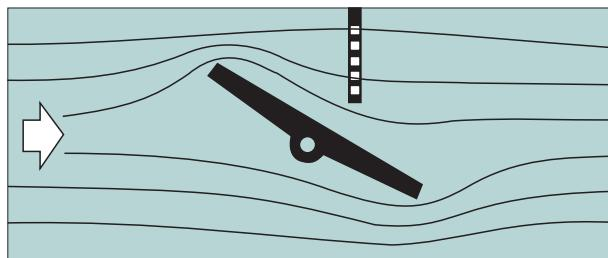
S-DISC design offers stable flow control, reduced dynamic torque, noise level and vibration. For more information see technical bulletin 2SL120.
