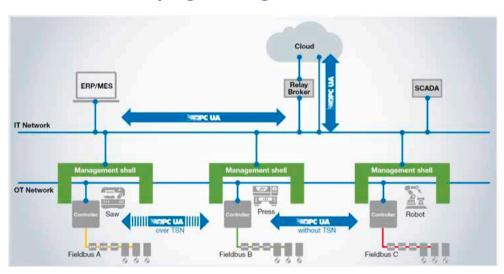
OPC-Unified Architecture (OPC-UA) is the innovative data exchange standard of the OPC Foundation. It ensures secure, reliable, and both manufacturer and platform-independent transfer of information that is not restricted or tied to any proprietary technology or manufacturer. OPC-UA allows access to any authorized application and to retrieve any information from anywhere and at any time.
