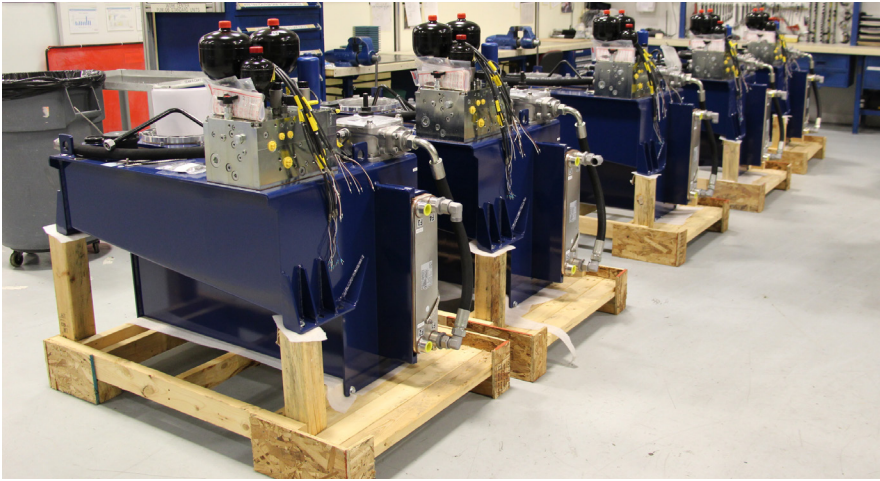
Hydraulic power units designed for use in a serial application can incorporate unique or specific features for the machine series.
