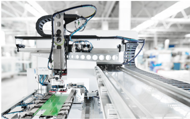
Separating circuit boards
