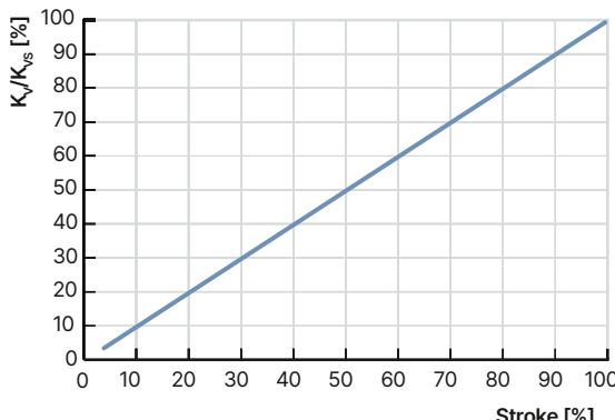
Linear flow characteristic - the  $K_{vs}$  values of the respective seat sizes can be found in chapter "6.2. Pressure range" on page 13.
