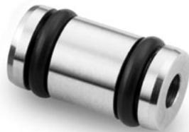
Slip-fit Pressure Connectors provide flowpath intra-connectivity between Parker IntraFlow™ fittings. Pressure Connectors are fully assembled with AS568B standard size 2-008 o-rings and are available in both standard and jumper lengths (for systems with flow requirements between non-contiguous fittings). Orifice is 1/8" and various elastomers are available.
