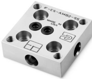
All Parker IntraFlow™ fittings are permanently marked with the part number, flow schematic and material heat traceability code for easy identification during assembly and when servicing in the field. 1/8" diameter internal flow paths are precision machined at the intersections to minimize dead volume. Slip fit counterbores with a lead-in chamfer retain intra-connecting pressure connectors.
