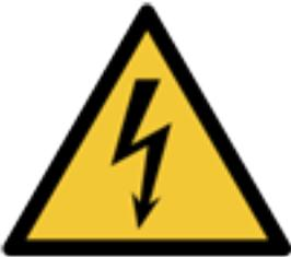
**ELECTRICAL HAZARD** - Hazards referring to electrical conditions such as high voltage. Refer to specific details listed next to symbol.
