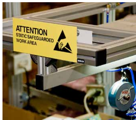
T-slotted aluminum framing systems are an outstanding construction system for lean workstations: The T-slot design lets you mount work instructions, tools, parts bins and fixtures anywhere along the frame, and the bolt-together construction means that you can easily disassemble and reconfigure them as your needs change.
