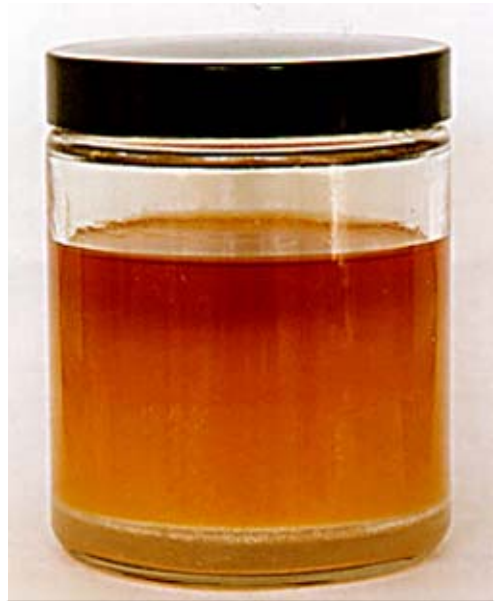
Figure 2 Dissolved, emulsified and free water in oil, with a biological contamination at the water interface.
