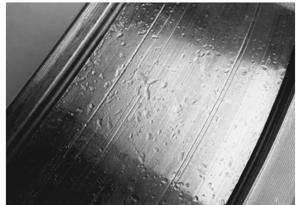
Fatigue wear results induced by pressure and accelerated by water in oil.
